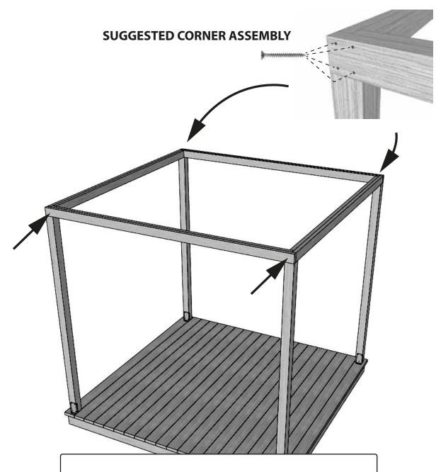
WE SUGGEST PRE-DRILLING WITH 1/16" DRILL BIT FOR THE WHOLE CONSTRUCTION.
