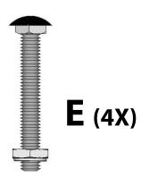
Bolts (E) are not required for 3"/80 mm beams
