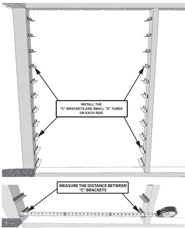
(Repeat this step for each board, it is possible that the boards are not all exactly the same length)
