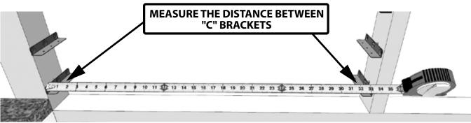
(Repeat this step for each board, it is possible that the boards are not all exactly the same length)
