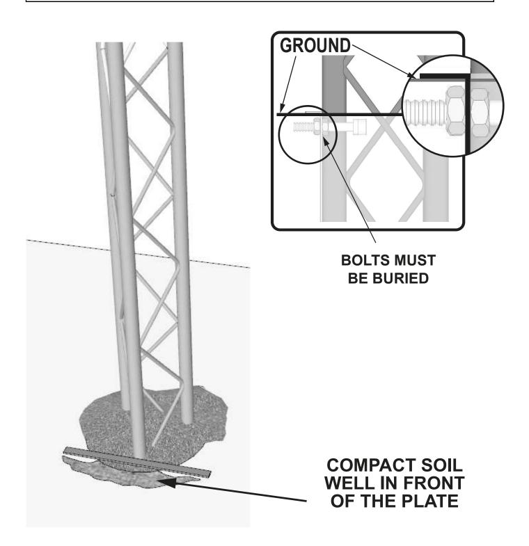
Standard 11' above ground. Possibility of adding an extension (item #: 10738) to have a maximum of 15' above ground.
