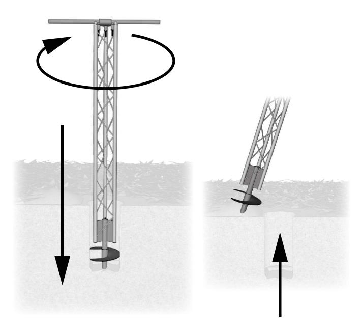
SCREW 6" AND REMOVE SOIL EACH TIME. REPEAT UNTIL PIECE (A) IS 8" IN ABOVE GROUND LEVEL.
