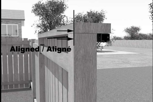
**Install the "Rail Assembly" on the 4" x 4" using 3½" wood screws (not included).
