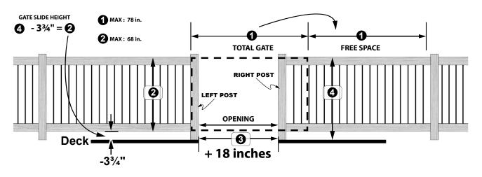
1 = Total gate / 2 = Height of sliding gate / 3 = Opening / 4 = Height of railing
