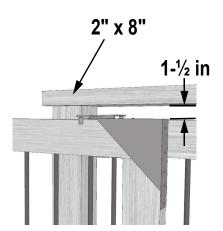
TO PREVENT INTERFERENCE TO "MECHANISM" LEAVE A SPACE OF ABOUT 1-1/2"
